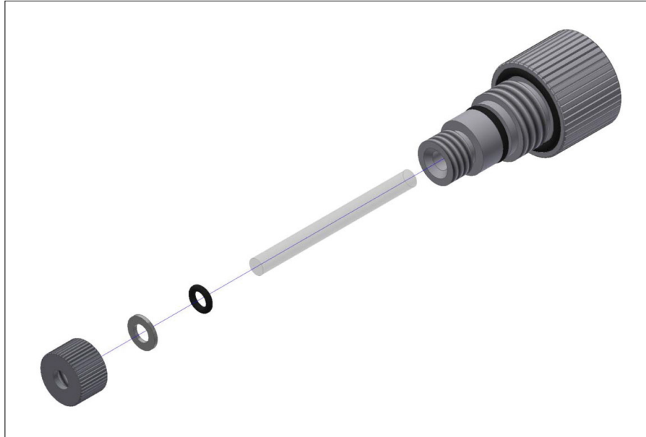
Figure 14 – Removing Quartz Rod from Remote Probe
