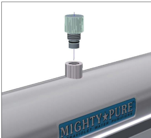
Figure 7 – Removal of Sight Port Plug
