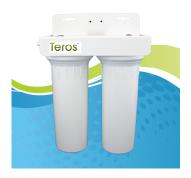
The Teros<sup>™</sup>2S UF uses our latest Gen2 hollow fiber membrane technology for exceptional bacteria, cyst and virus reduction and our AquaMetix® filter for unequaled chemical reductions. The Teros<sup>™</sup>2S is a twin system capable of delivering >0.5 gallon per minute flow rates without the need of a storage tank.
